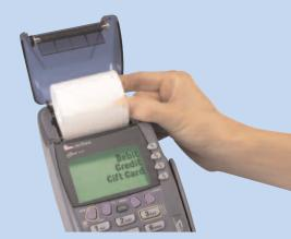
A "clam shell" printer facilitates drop-in loading, virtually eliminating paper jams.
